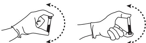
c. Analyze immediately after mixing. Subsequent analyses during this test period may be performed by inverting the vial 5 times prior to instrument analysis.
