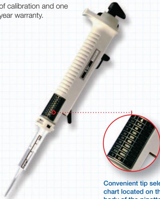
Convenient tip selection chart located on the body of the pipette.
