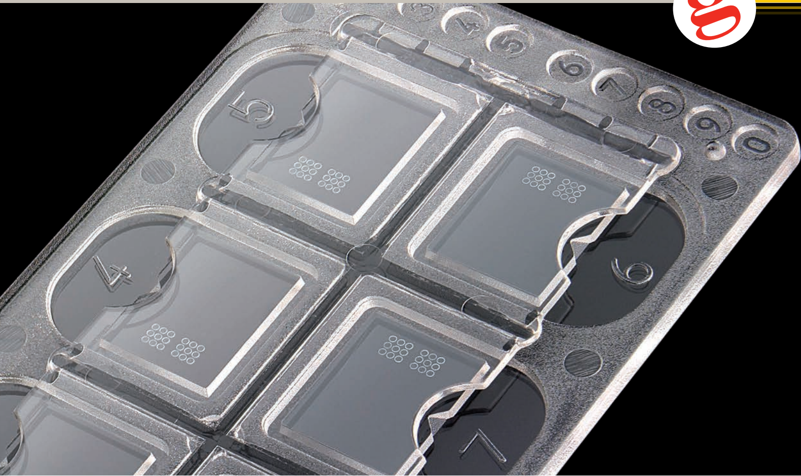
3805 — Quick-Read Precision Cell urinalysis microscope slide
