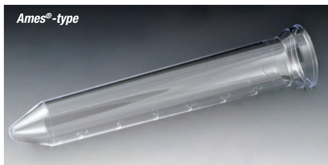
112017 — Ames®-type urine centrifuge tube
